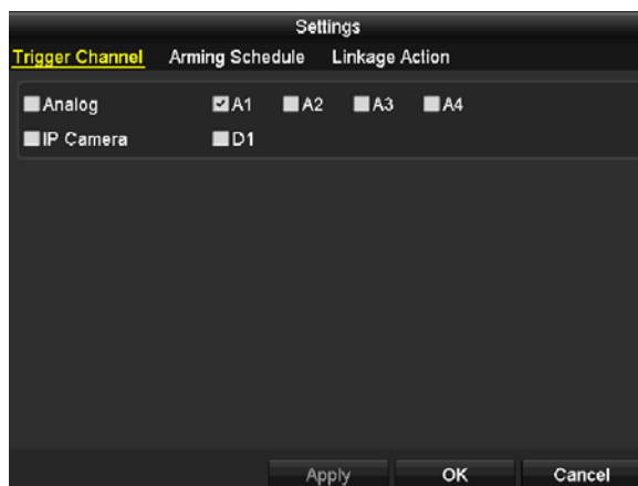
Figure 8.15 Set Triggering Channel of VCA Alarm
